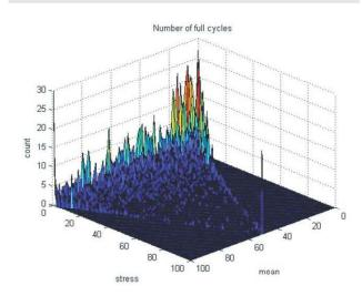
Projections of 3D ESS Stress Chart give histograms of Cycles Vs DoD swings
